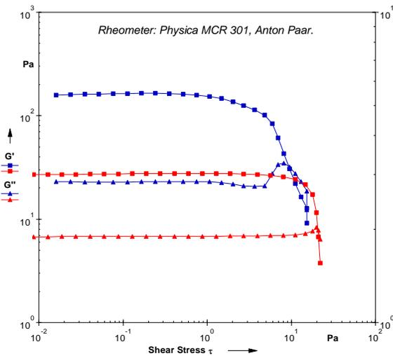
Figure 3: Stress amplitude sweep of 1% active Betafib<sup>®</sup> (blue) vs. 1% active xanthan (red) in water at 20 °C.
