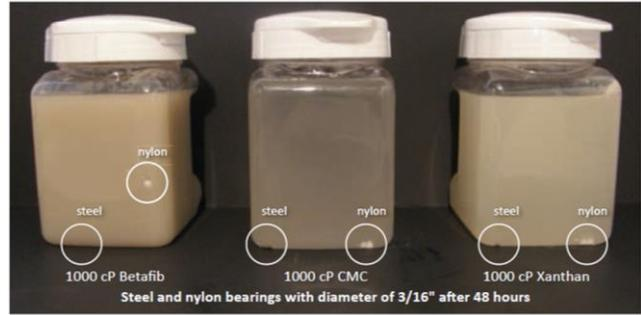
Figure 4: Comparison of particle carrying properties of Betafib<sup>®</sup> MCF, CMC and xanthan.
