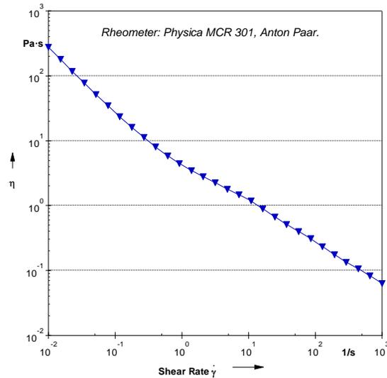
Figure 2: Flowcurve for 1% active Betafib<sup>®</sup> microcellulosic fibers in water at 20 °C.
